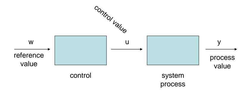
assumption: undisturbed operation  $\Rightarrow$  process value = reference value
