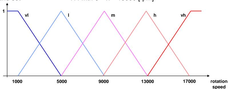
industrial drill machine → control of cooling supply
